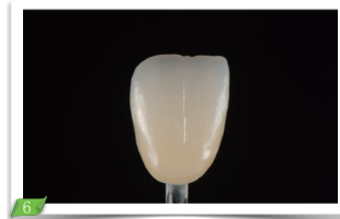
6 Complete the sintering according to the recommended sintering curve, the restoration after sintering presents a beautiful natural feeling.
